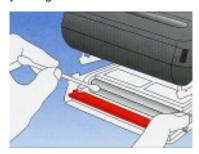
Close the bar. Reload the film; the top picture will be lost, and will advance into the storage compartment. The picture counter will reset to 10 and will miscount the rest of the pack.
